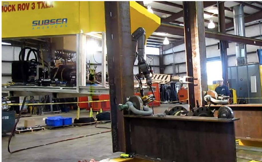
Above shows trials conducted on client WI PLET project. The project involved the removal and replacement of an existing WI PLET and installation of a flexible jumper. One of the problems that was encountered was the need to remove old rigging left subsea on the PLET for 5 years. A real size mock up of the back end of the PLET was built and the mock ROV was used to prove the methods of split pin removal from the shackles then open the shackles, remove and replace.
