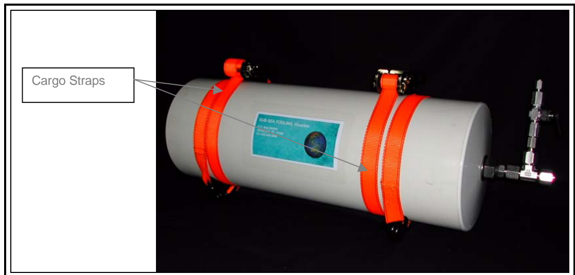
Fig 2.1.3 Reservoir Mounting Hardware
