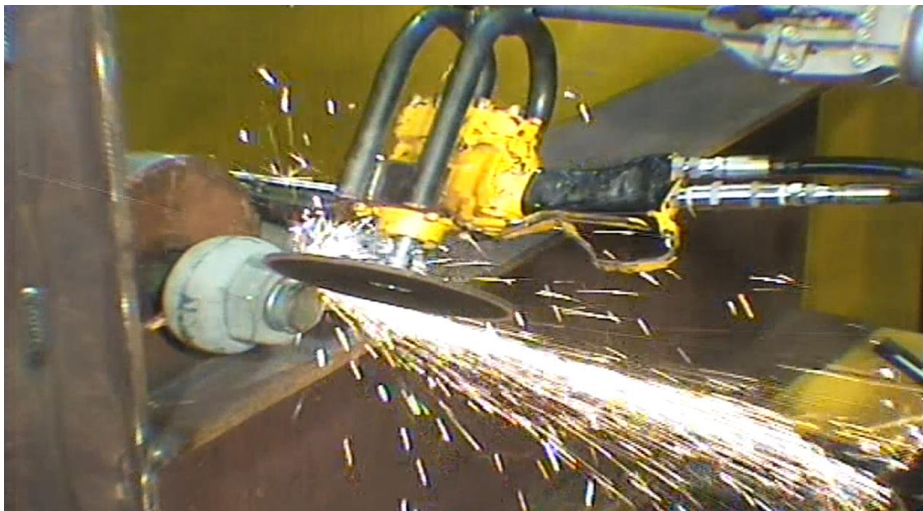
Pilot view cutting split pin
